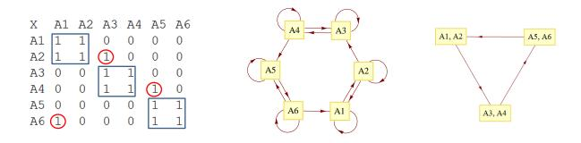
**Fig. 2**: Near-decomposability and modularization in a circular system: activity dependence in binary terms with modules in blue and interfaces in red (left), system graph of all elements (middle) and of simplified modules (right).
